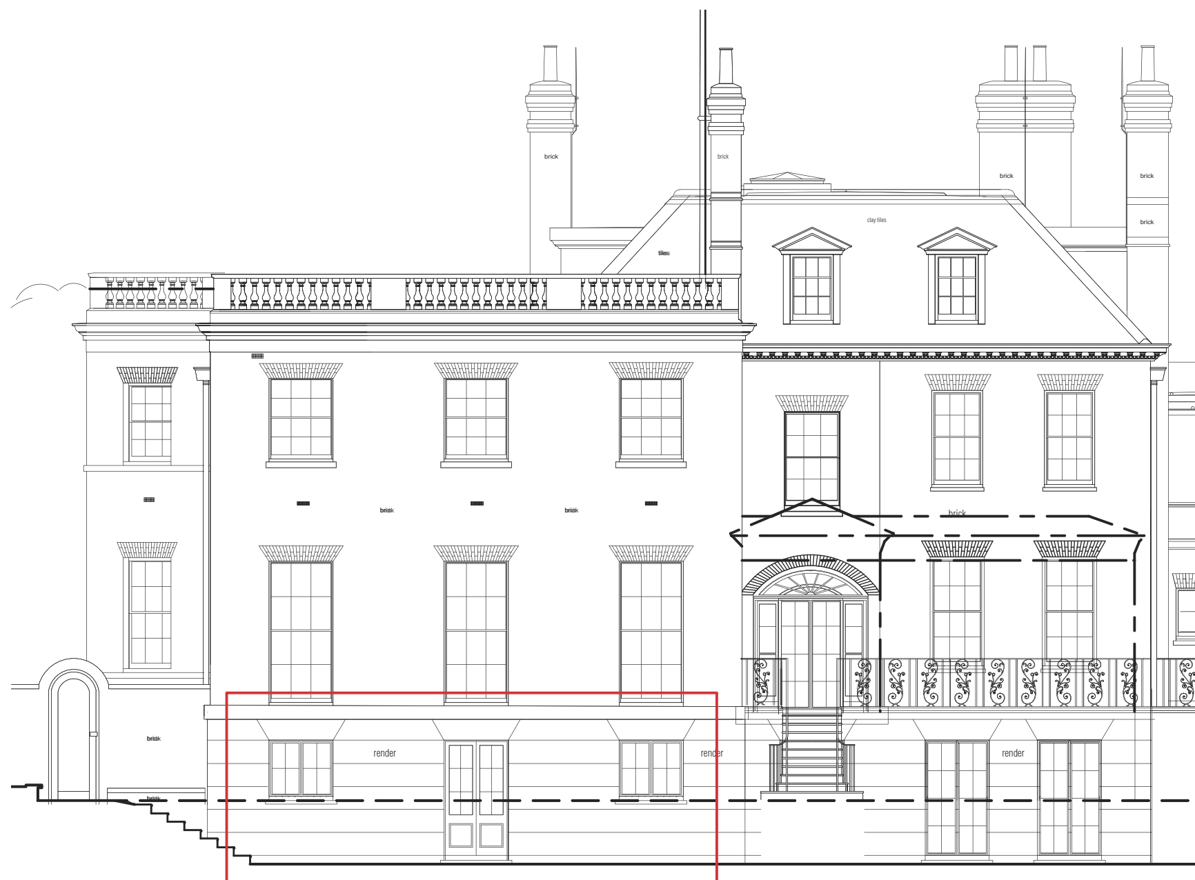
PROPOSED DOOR (1no.) ALTERNATIVE 3 As alternative 1 + stile width increased further, base rail reduced in height to balance the width of the stiles / rails. Glazing unbalanced in context of elevation.
