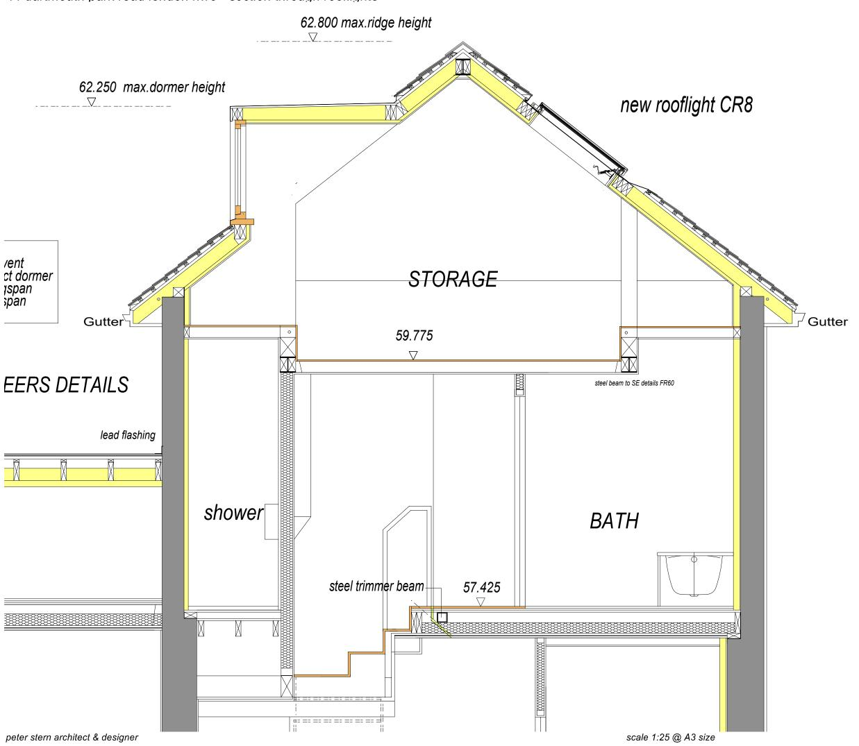
MAIN PITCHED ROOF reconstructed to new pitch,37 degrees a onto battens and counter battens onto K membrane, onto new rafters. 125 Koolth with 32.5 Kingspan Kooltherm K18 with supporting structure to engineers design
