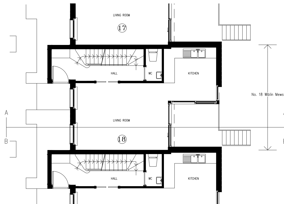
Ground Floor Plan Scale 1:100
