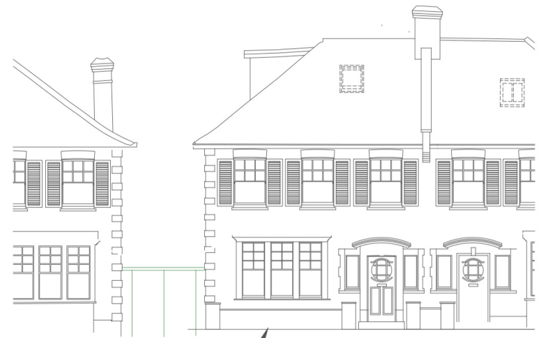
Construct dwarf brick wall with pillars and freestone copings
