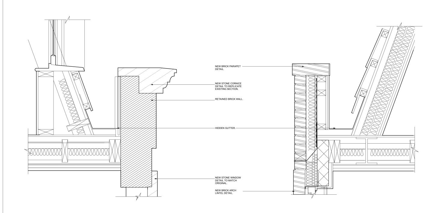
de52 Detail Showing Block E Parapet Cornice and Mansard Roof Junction  $_{1:5\ @\ A1,\ 1:10\ @\ A3}$
