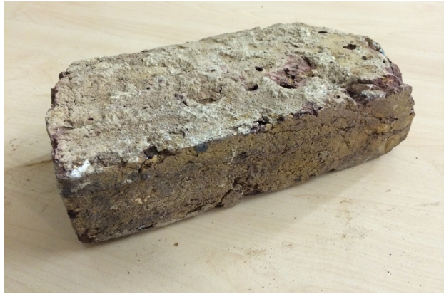
Proposed Brick - Yellow skinned red brick 'seconds'. To be 'sooted' to match existing facade and repainted below soldier course datum in line with the existing elevation.
