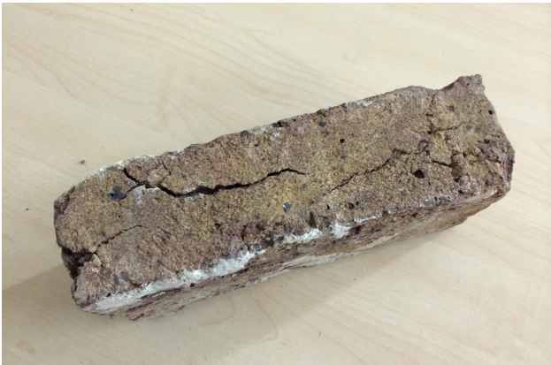
Existing Brick - Yellow skinned red brick 'seconds'. Existing soot and paint visible.
