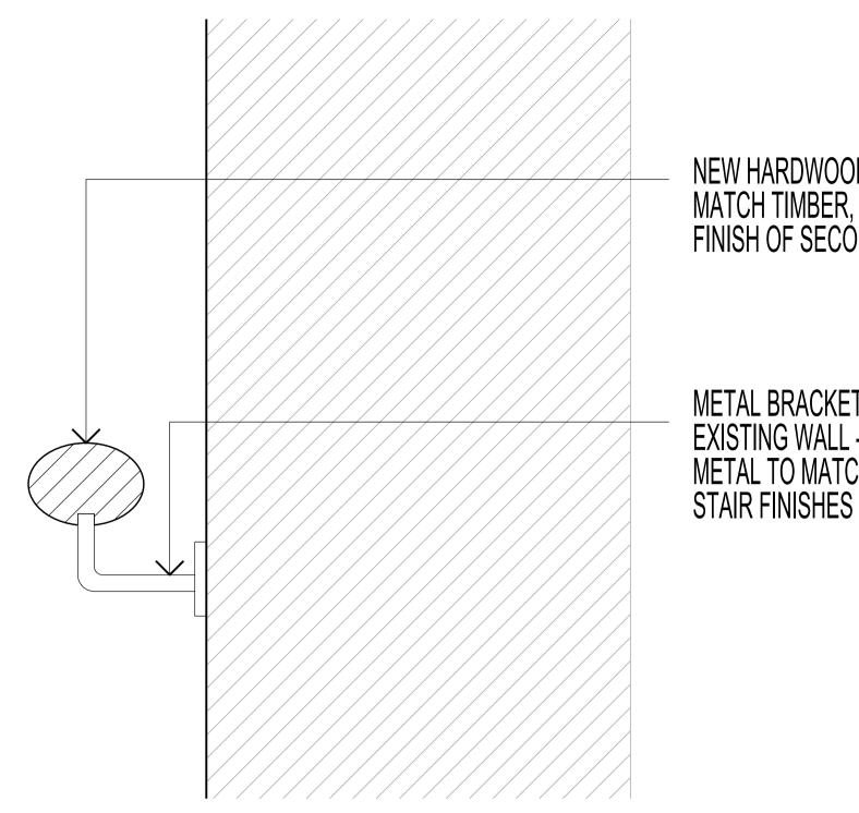
NEW HARDWOOD HANDRAIL TO MATCH TIMBER, PROFILE AND FINISH OF SECONDARY STAIR
