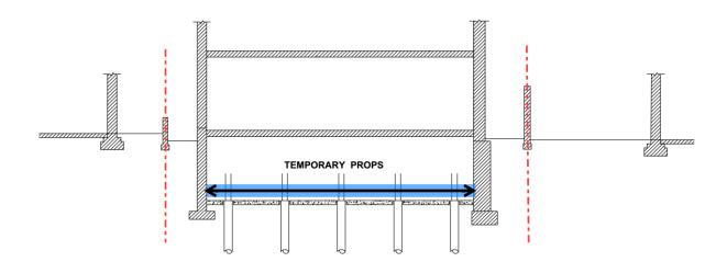
4. Once the temporary props are in place, carefully remove the existing basement slab. Locally excavate ground around the installed piles and carefully break down the top of piles to the required cut-off level using hand-held pneumatic breakers, leaving top of reinforcement to form an anchorage into the new slab.
