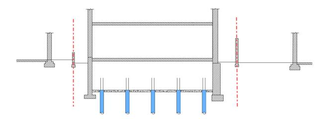
3. Install temporary lateral props to the base of all retaining walls above the existing basement slab level.
