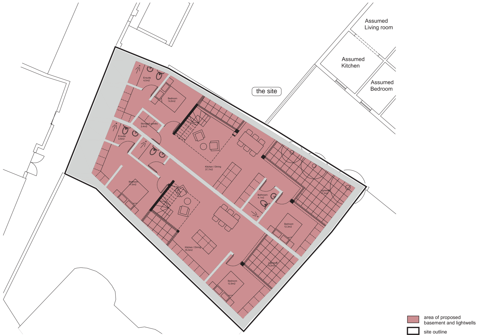
Fig 19 Plan of the proposed lower ground floor (Martin Evans Architects, dwg. no. STRB-PL-GA-00, 14/02/2018, Rev-)
