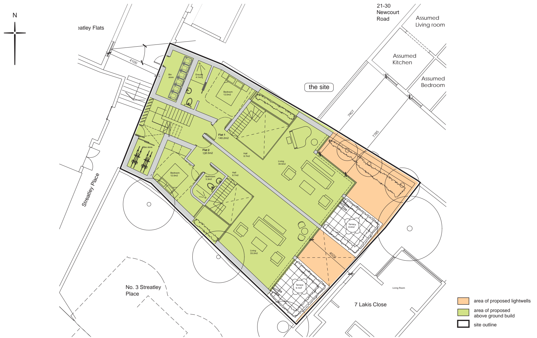
Fig 18 Plan of the proposed ground floor (Martin Evans Architects, dwg. no. STR-PL-GA-01, 14/02/2018 Rev-)
