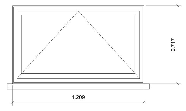
We propose replacing the existing window with a single glazed top hung casement with a clear double glazed and laminated glass, thus allowing us to remove the external security bars. Window frame and casment to be painted white to match adjacant windows and frames
