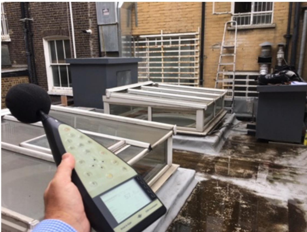
View of sound level meter measuring background noise near residents at rear, on flat roof.
