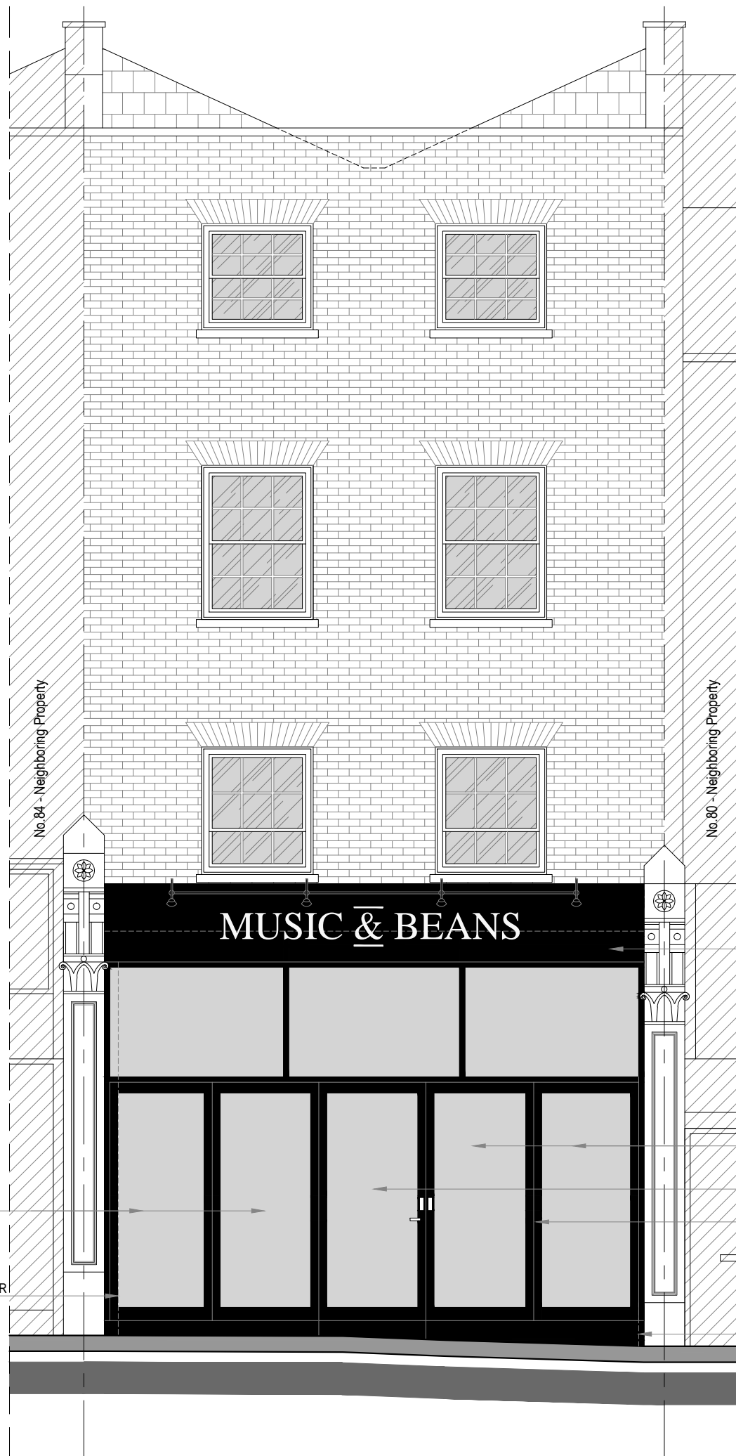
PROPOSED SHOPFRONT - FRONT VIEW scale 1:50
