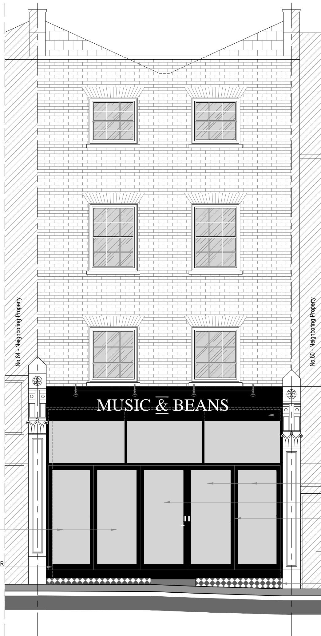
EXISTING SHOPFRONT - FRONT VIEW scale 1:50
