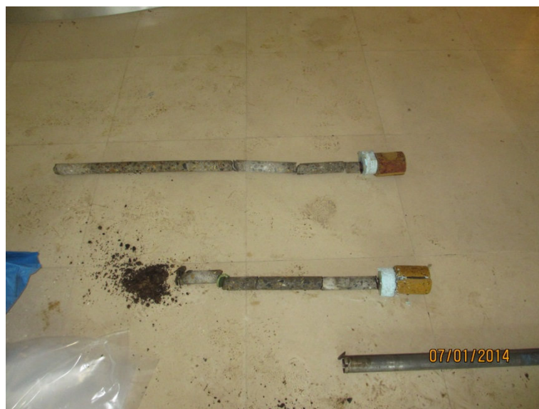
Photo 02 – Typical Cores (Low Level top & High Level bottom)
