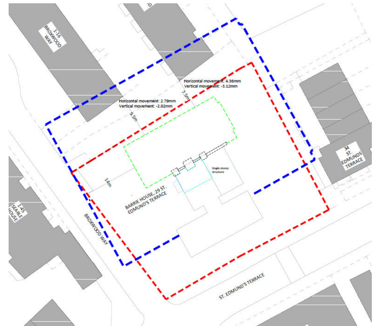
Figure 21 CGL Ground Movement Assessment Summary
