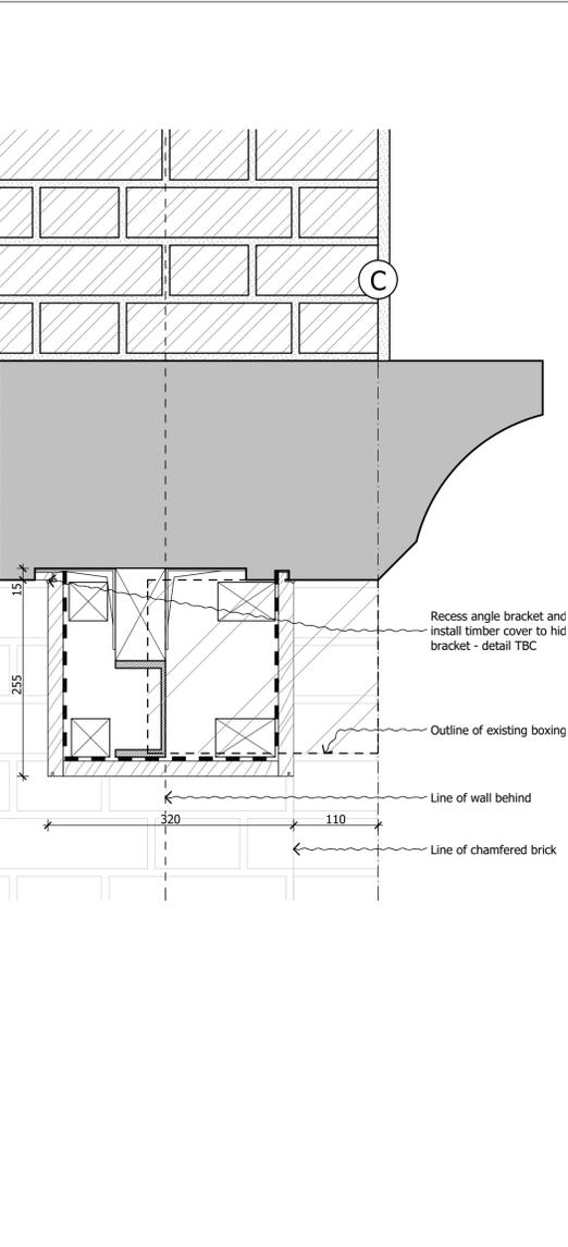
6 SCALE 1:5 @ A1, 1:10 @ A3 SECTION DETAIL - CANTILEVERED STEEL BEAM
