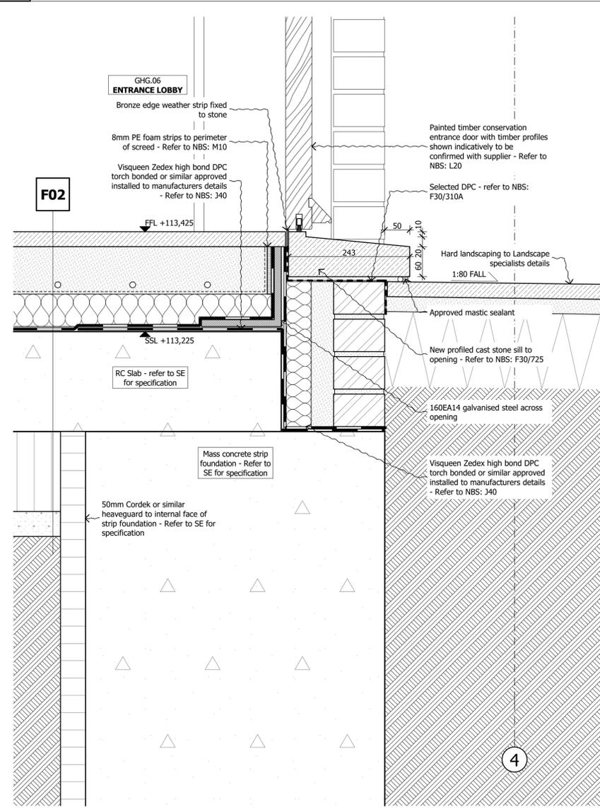
4 SCALE 1:5 @ A1, 1:10 @ A3 SECTION D-D DETAIL - BELOW GROUND NEW EXTENSION DOOR SILL
