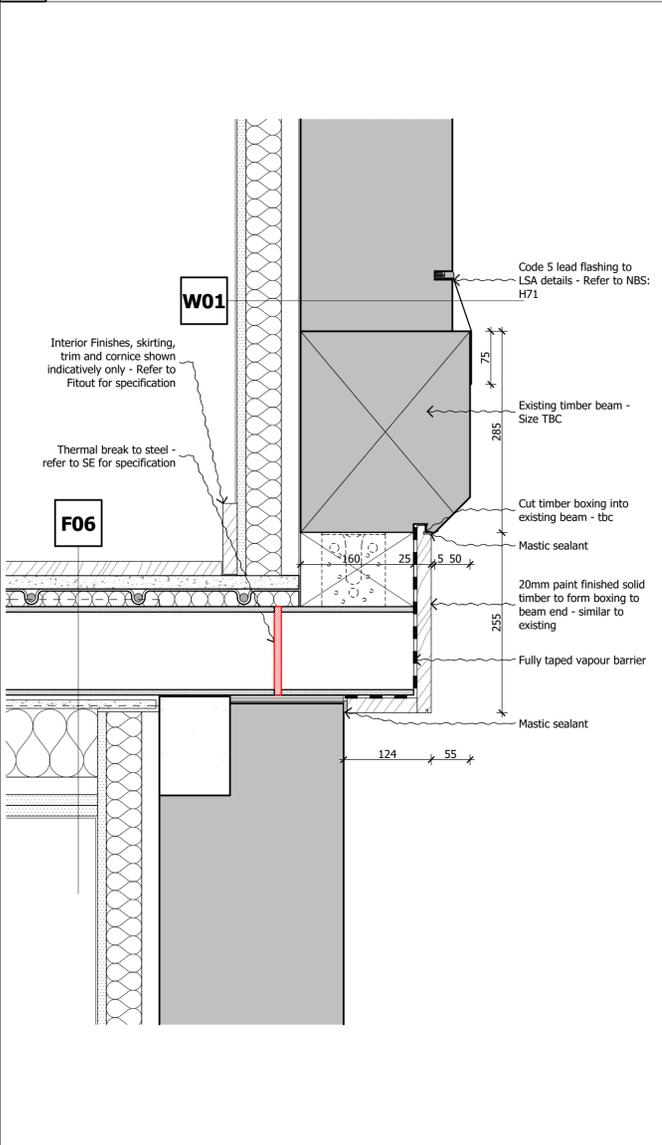
3 SCALE 1:5 @ A1, 1:10 @ A3 LONG SECTION DETAIL - CANTILEVERED STEEL BEAM
