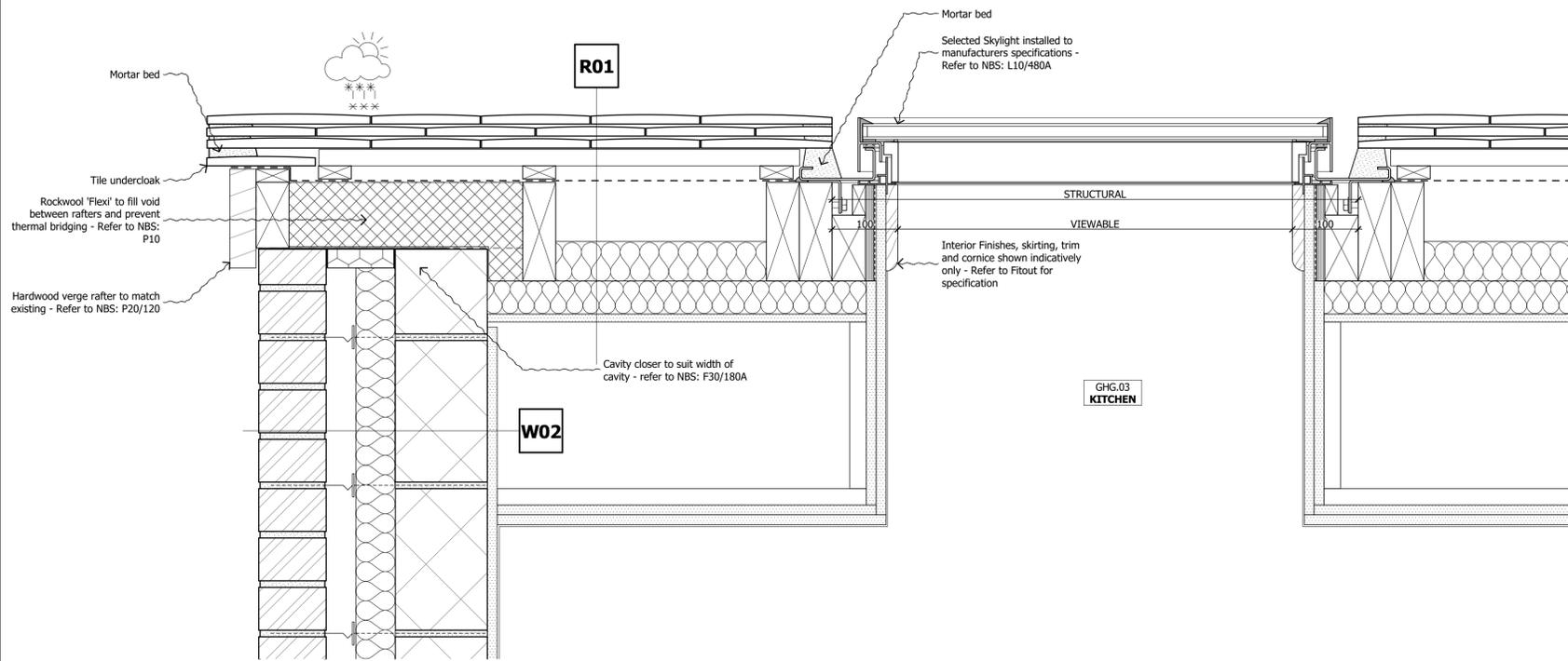
1 SCALE 1:5 @ A1, 1:10 @ A3 SECTION D-D DETAIL - SKYLIGHT AND NEW EXTENSION VERGE
