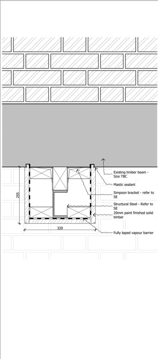
5 SCALE 1:5 @ A1, 1:10 @ A3 SECTION DETAIL - CANTILEVERED STEEL BEAM
