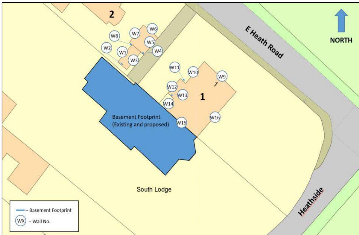
Figure 5: Ground Movement Assessment Wall Location Plan
