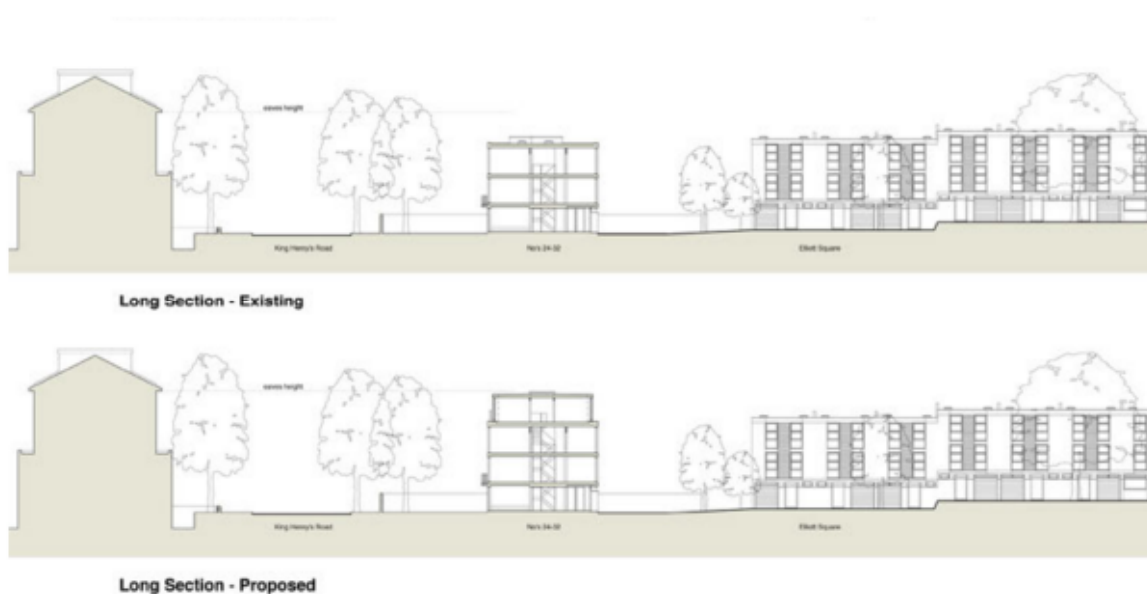
7. Existing and proposed long section through Elliott Square showing relationship to larger houses on King Henry's Road
