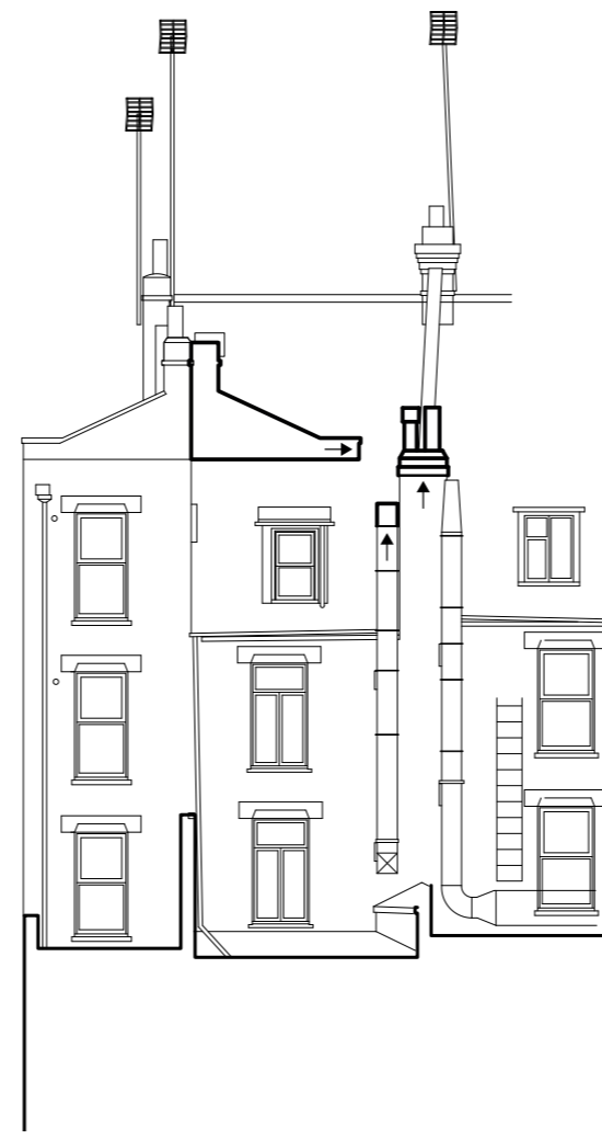
3. Mirrored roof extended together with chimney and commercial extraction duct.
