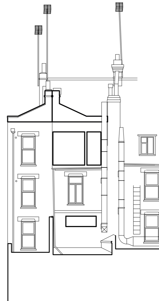
4. New glazing installed.
