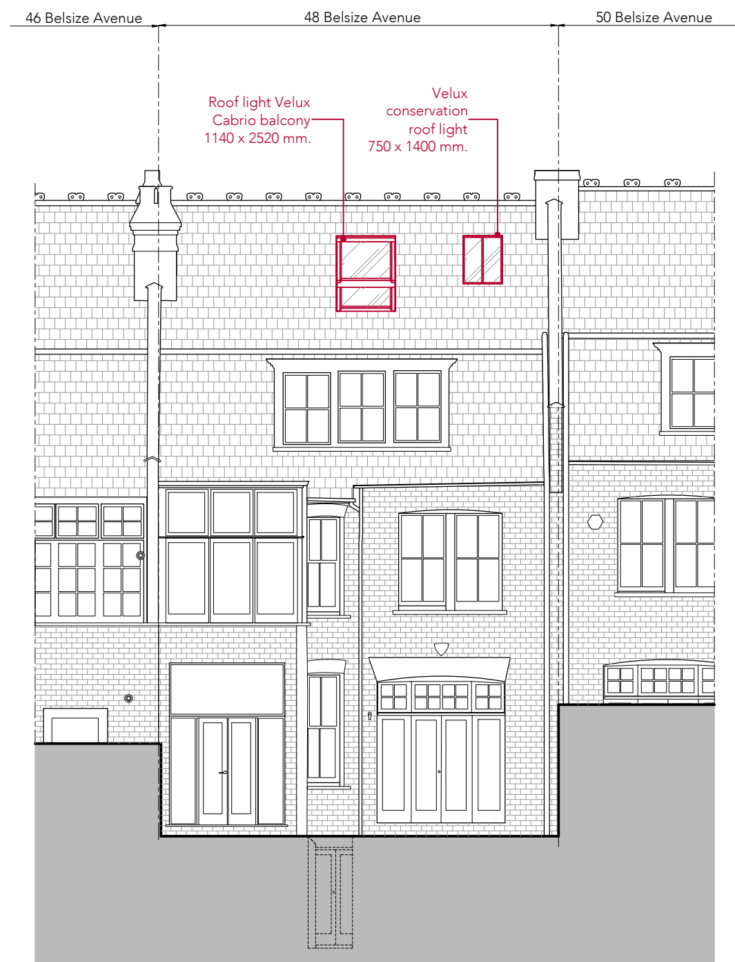
2 Proposed Rear Elevation scale 1:100
