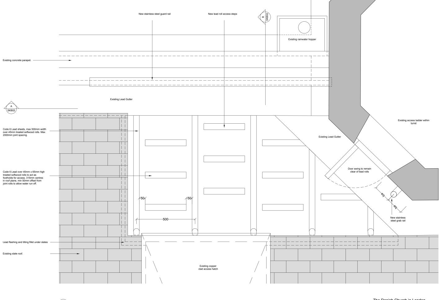
Roof Access Plan - New access steps to existing maintenance hatch Scale 1:10
