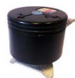
Geophone on small tripod base
