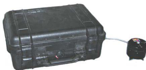
Example of Vibration Monitoring Unit in Weatherproof case and external geophone
