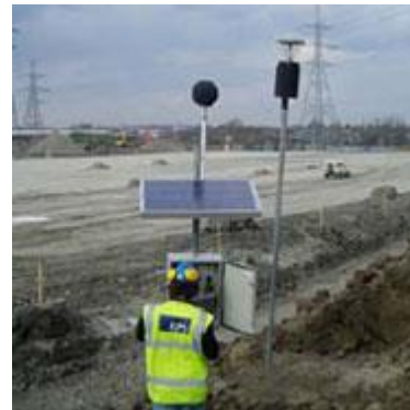
Examples of a Dust Monitoring Unit and Placement on Site
