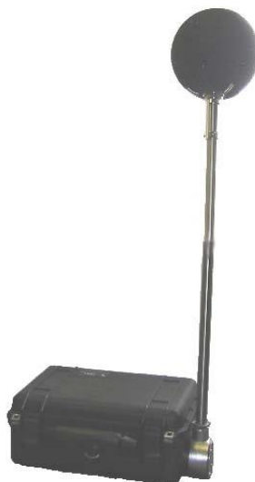
Example of Sound Meter within Weatherproof case and External Microphone
