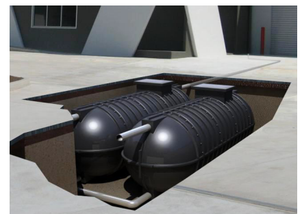
Low level interconnecting pipework
