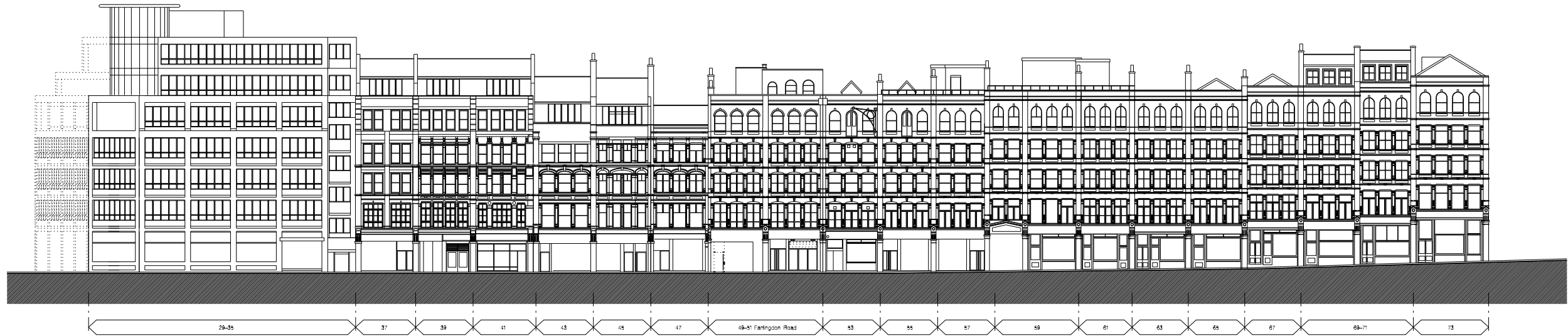
① EXISTING FARRINGTON ROAD CONTEXT ELEVATION
