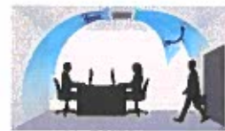
Comfortable air conditioning by preventing direct blowing of cold air and by providing swinging air flow simultaneously
