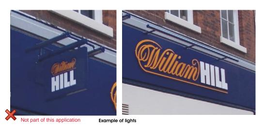
The illumination to the signs is very local to the sign only using LED trough lights. The lights are small at only 50mm height. The lighting will be positioned to shine toward the fascia and down and not up towards the flats above.
