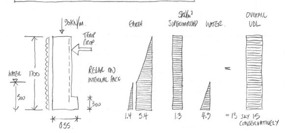
REGAMNIC WALL ANALYSED AS A SIMPLY SUPPORTED BEAM WITH NO FIXITY AS THE LASE WITH OVERGIVENING MOMBRUT RESISTED BY THE TEMPORARY PROPPING. A NOMINAL WATER PRESSURE IS INCLUDED BUT IS UNIVERYTO BE REPUSTIC AS THE REPAINING WALL WILL BECOME FULLY PROPPED BY THE RAFT FOUNDATION SOON AFFER COMPLETION. LATTACKL FONCES HAVE BEEN WOULED OUT IN TEXLA USING 0 = 33° (SCE SHEET RAFE 11) IN SIMPLE TOWNS. THE PROPRED WALL CAN BE IDEALUSED TO A SIMPLY SUPPORTED BEAM WITH A UDL OF LESS THAN IS KN/M
