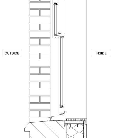
**02** Section Through Typical Traditional Timber Sliding Sash
