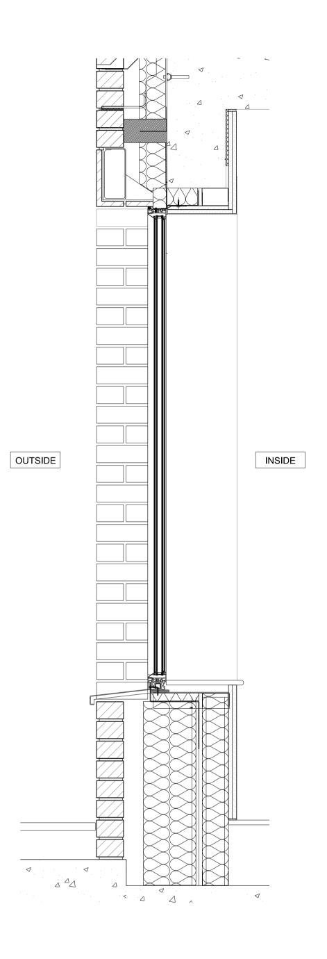
**02** Section Through Typical Aluminium Fixed Window 1:10
