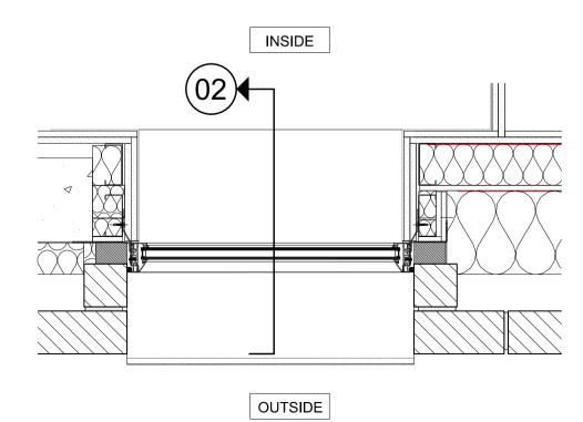
Plan of Typical Aluminium Fixed Window
