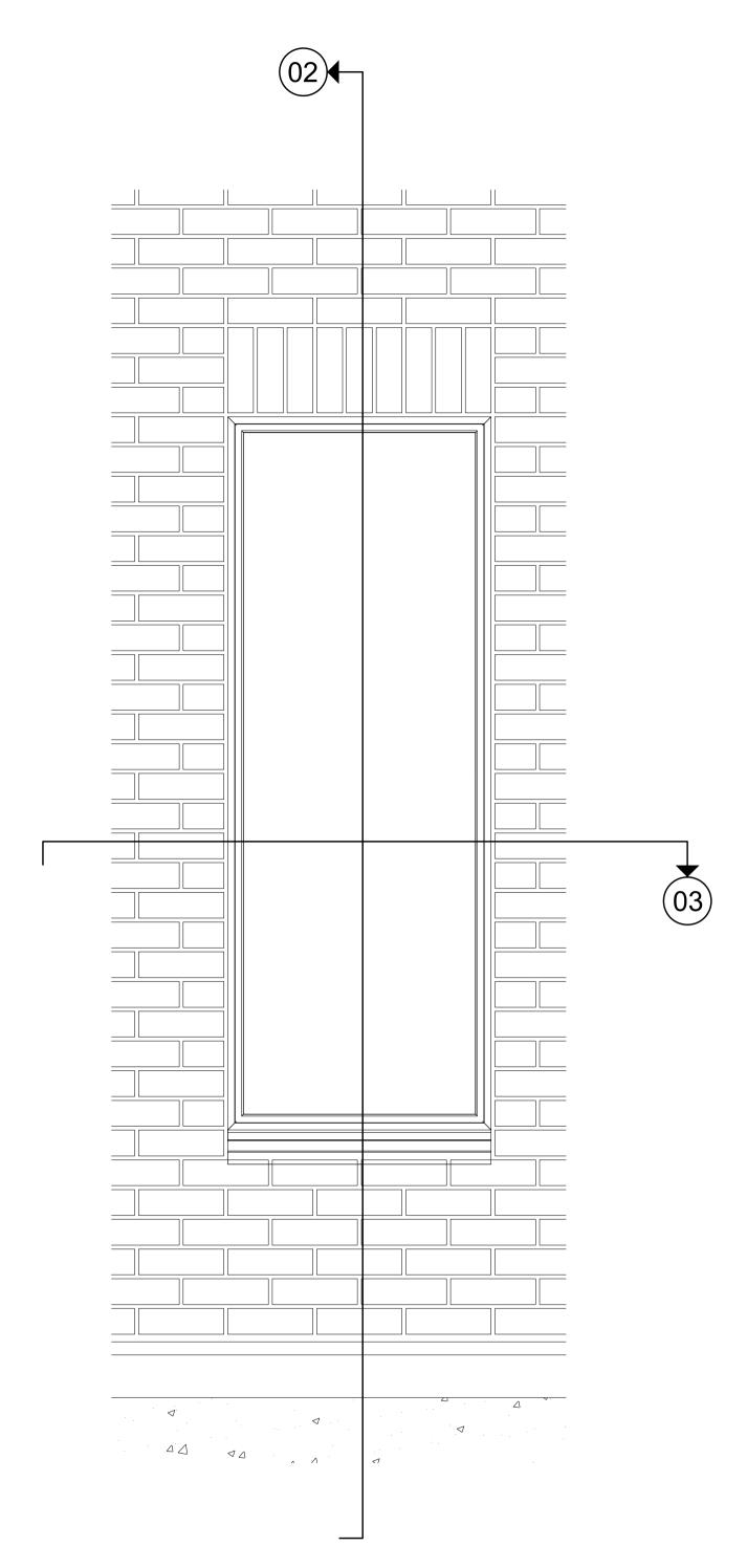
**01** Elevation of Typical Aluminium Fixed Window 1:10
