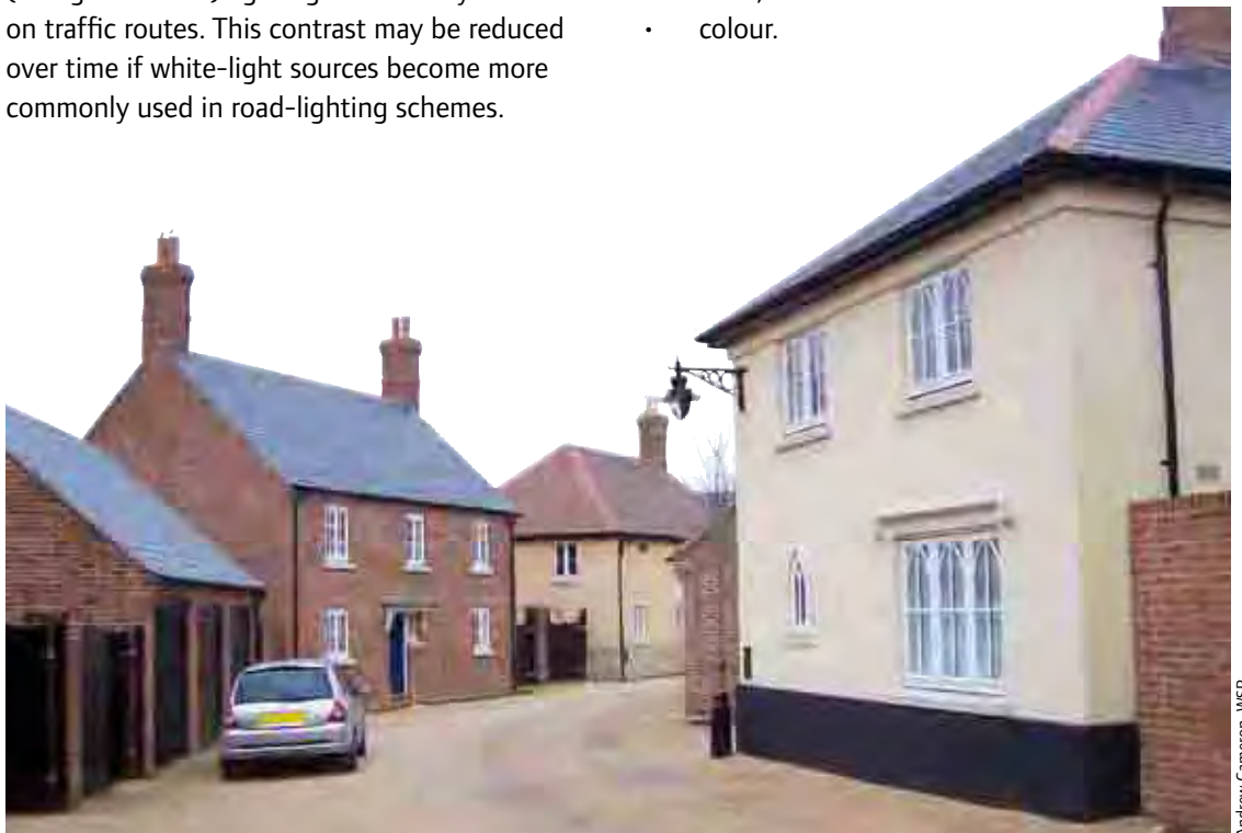
Figure 10.3 Street light mounted on a building.
