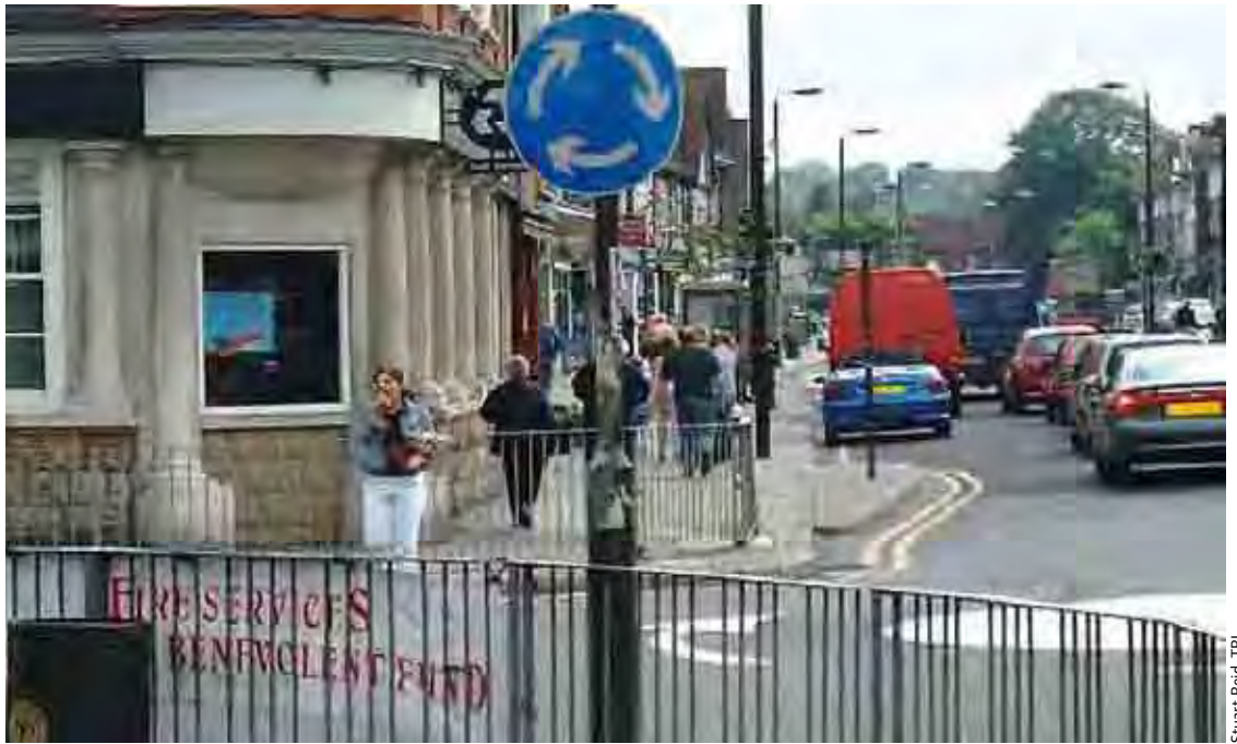
Figure 10.2 Guard railing blocking pedestrian desire line - note the pedestrian in the photograph has walked around it.
