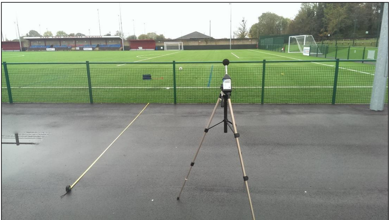
Figure 9: Impact noise measurement arrangement
