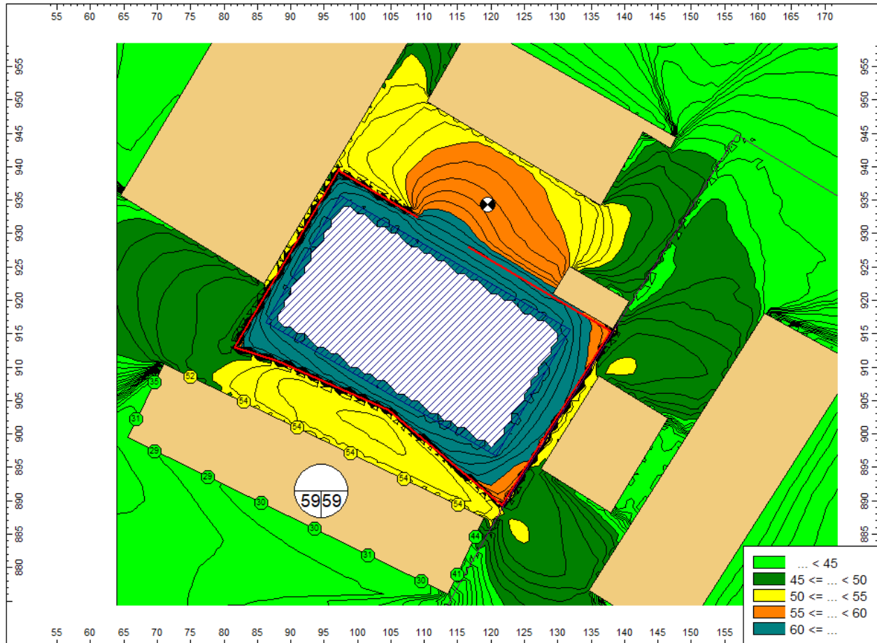
Figure 7: Predicted AGP Noise Emission (1.5 metres above the ground).
