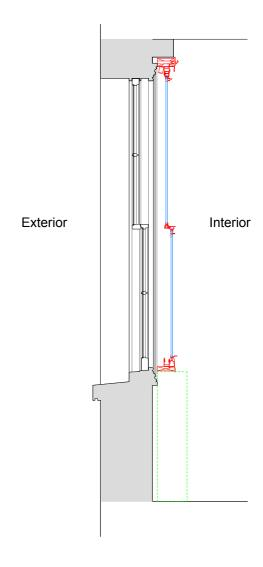
Plan Section B-B with Secondary Glazing Installed Scale: 1:10
