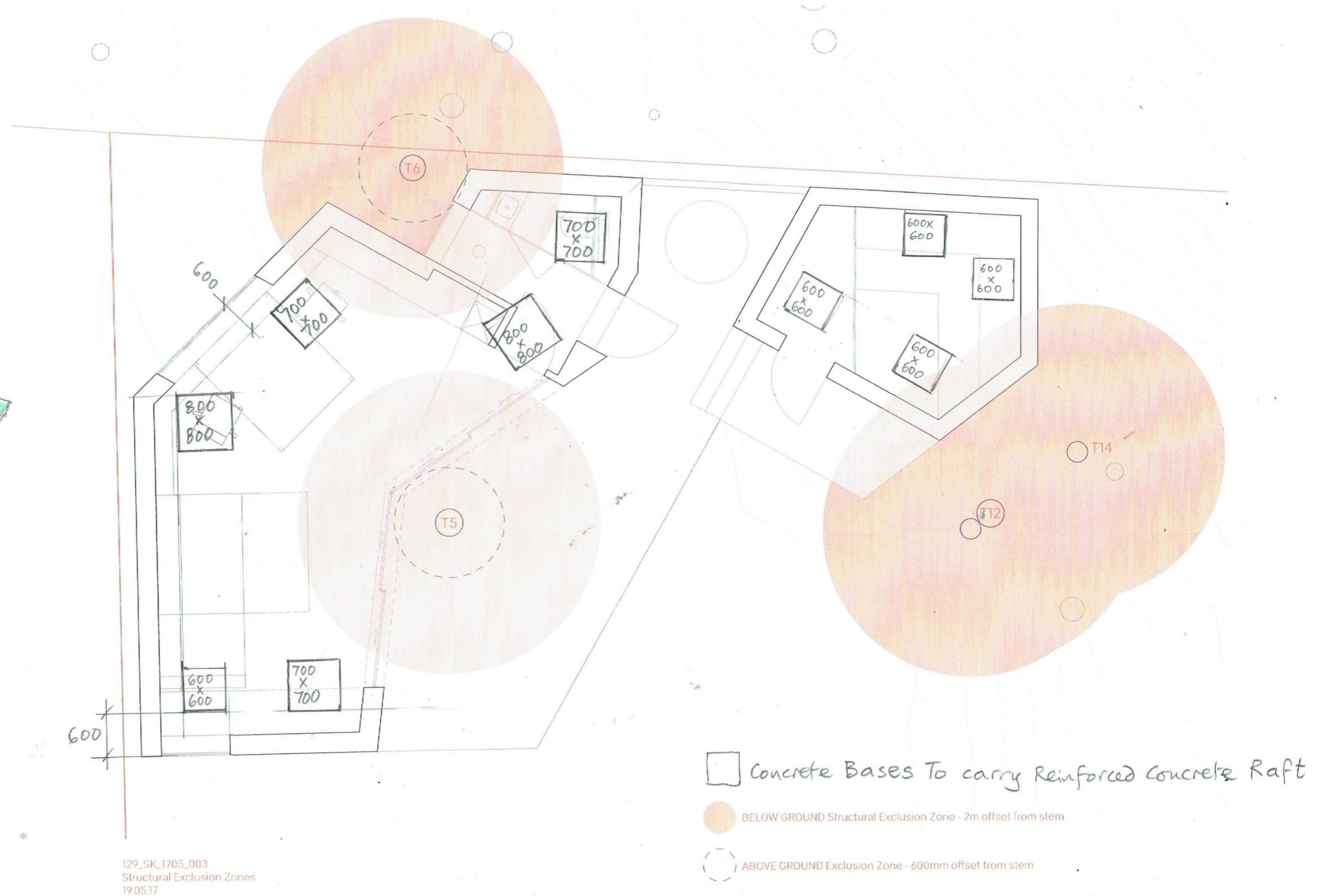
2. Structural sketch of garden room suspended raft slab and mini-pile footings: mini-pile locations to avoid root protection zones.
