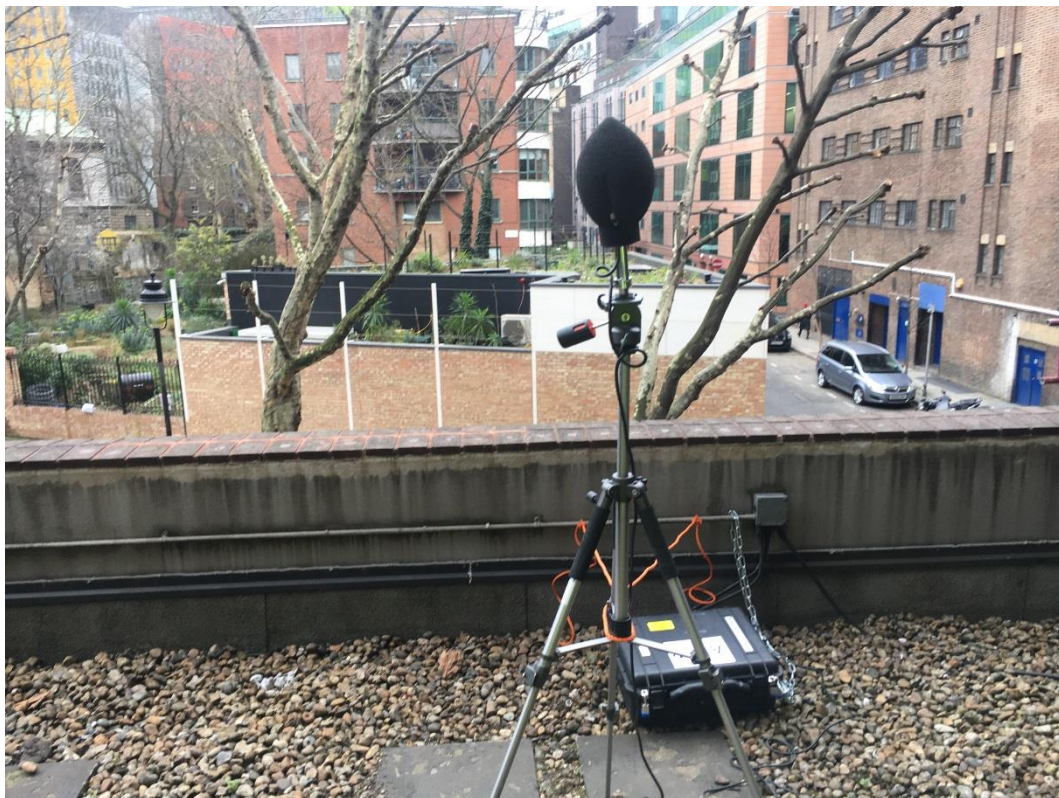
Figure 4: Unattended noise logger on the 1 st Floor Podium
