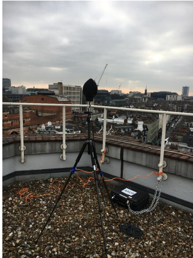
Figure 3: Unattended noise logger on the 7 th Floor Roof
