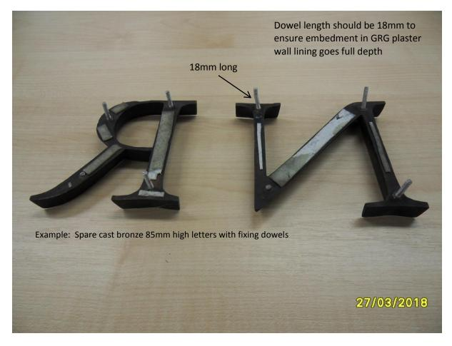
The bronze letters for the Piggott Room sign will be provided with 3mm diameter dowels for attaching to the GRG plaster wall face. Small holes will be drilled in the plaster for the dowels to be fixed using appropriate adhesive. This fixing method has been used successfully elsewhere in the building – see following photos of 'Philatelic Collections' sign in Front Hall on UGF.
