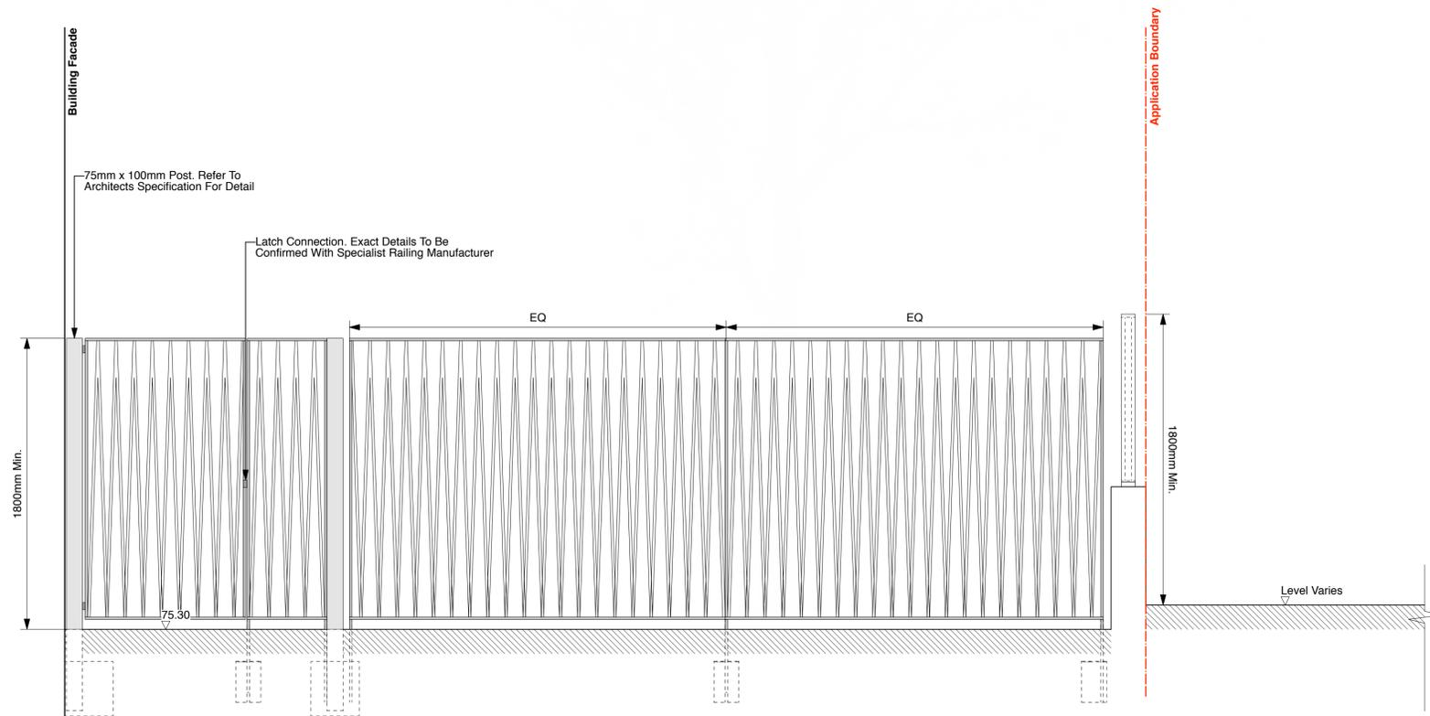
**Gate & Railing Elevation**
