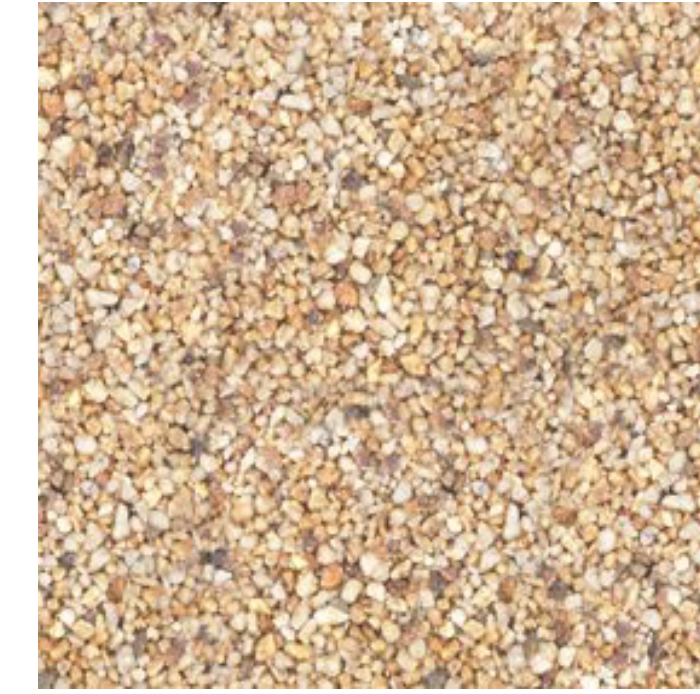
Typical Image Of Resin Bound Aggregate Surface (P6) Scale: Not To Scale
