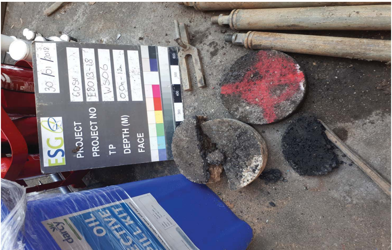
WS06 Concrete core
