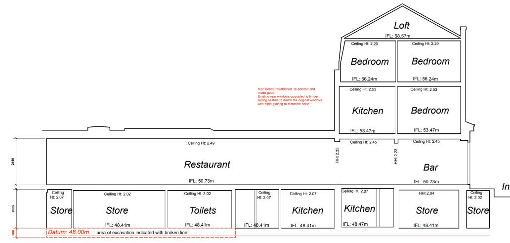
**Section B-B: Existing** scale 1.50 @ A1 (1.100 @ A3)
