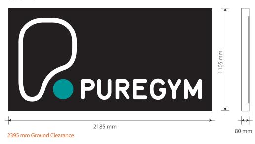
ITEM 02 (Qty 1) Projecting sign with lightbox 30mm trim double sided complete with acrylic panels with applied vinyl fixed into column fascia cladding panels Scale 1:20
