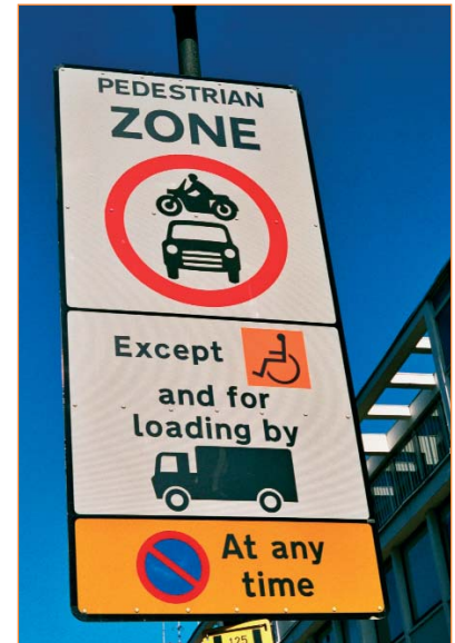
Combined vehicular signs to reduce clutter
