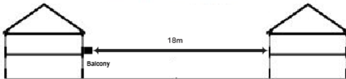
Figure A: 18m separation distance measurement
