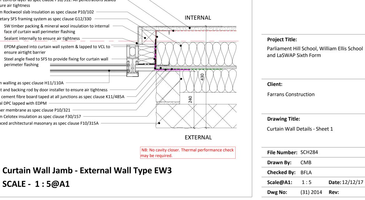
NB: Curtain wall perimeter flashing is non-loadbearing.
