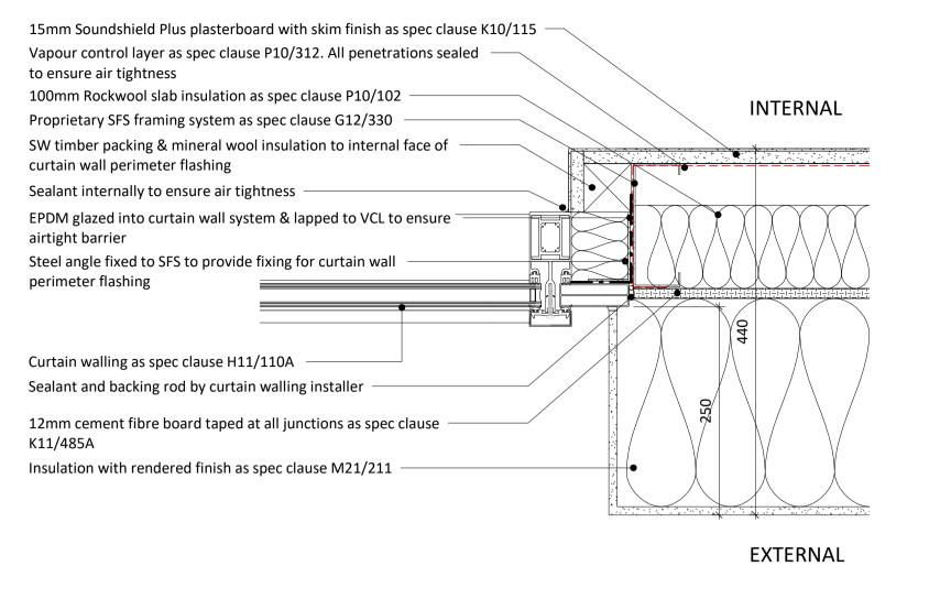
**Curtain Wall Jamb - External Wall Type EW2** SCALE - 1:5@A1
