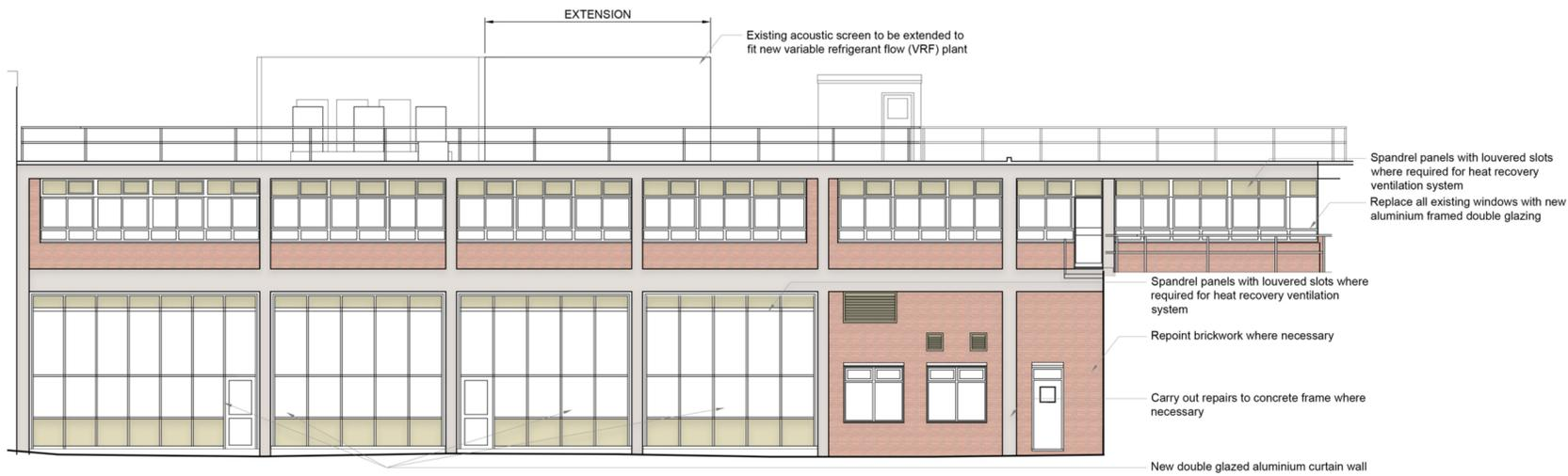
3 Proposed E7: internal west elevation
