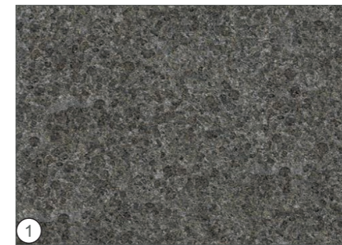
1 Granite corduroy paving to steps Supplier: Hardscape Product: Granite Colour: Crystal Black Finish: Flamed
