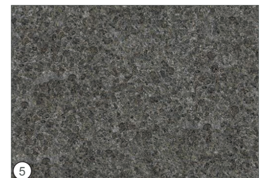
5 Granite corduroy paving to steps Supplier: Hardscape Product: Granite Colour: Crystal Black Finish: Flamed
