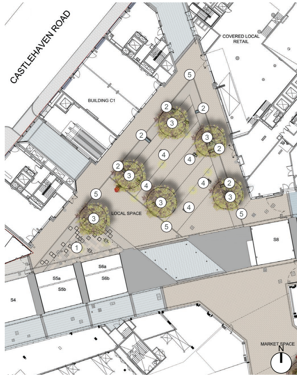
2 Granite seating with polished top and split sides
