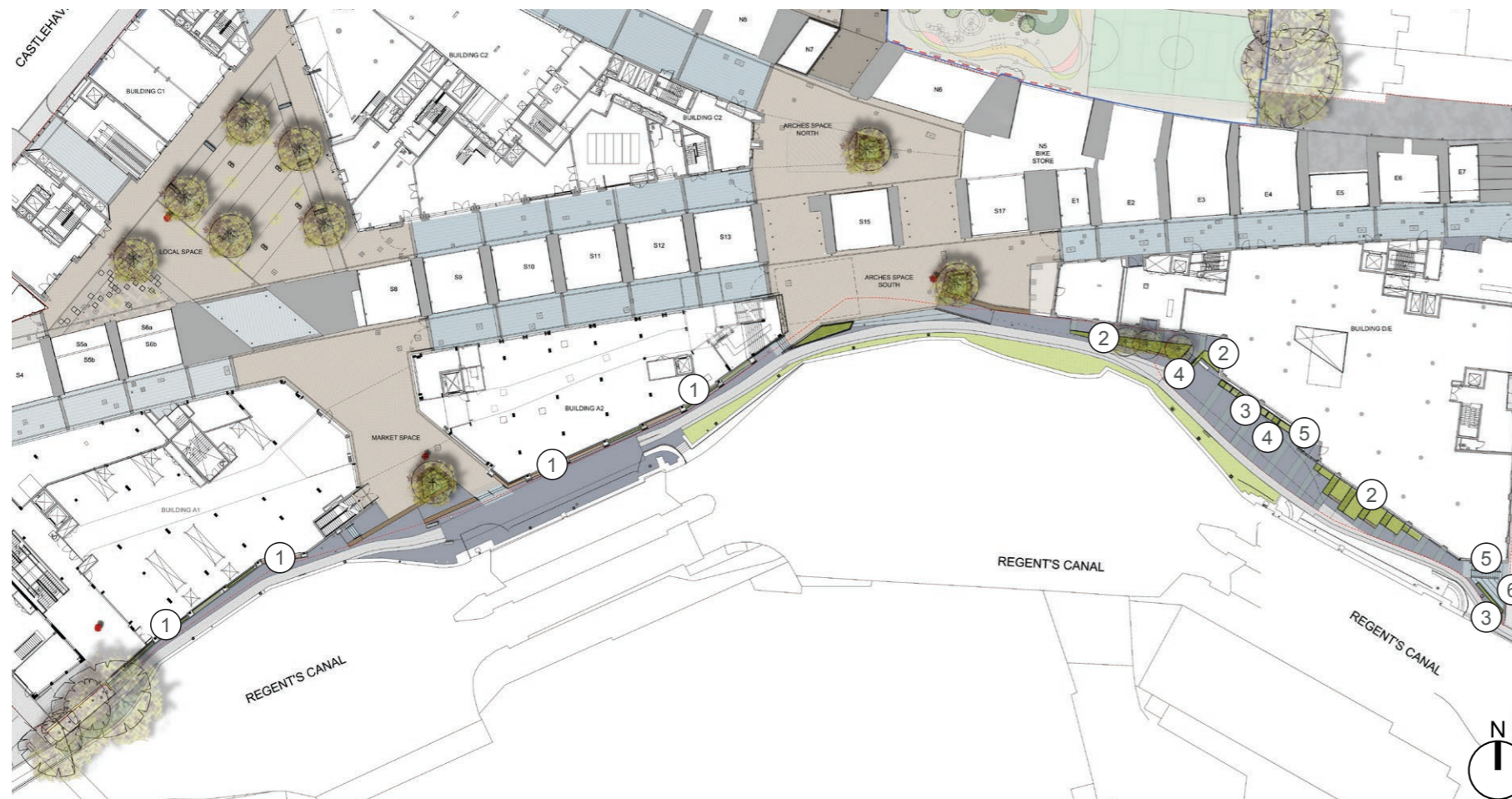
2 RAL 5004 Raised metal planter with integrated timber seating Supplier: Kinley Product: Perimeta planterline Finish: Powder coated Colour: Ral 5004 'Black Blue' (Corten steel finish shown)
