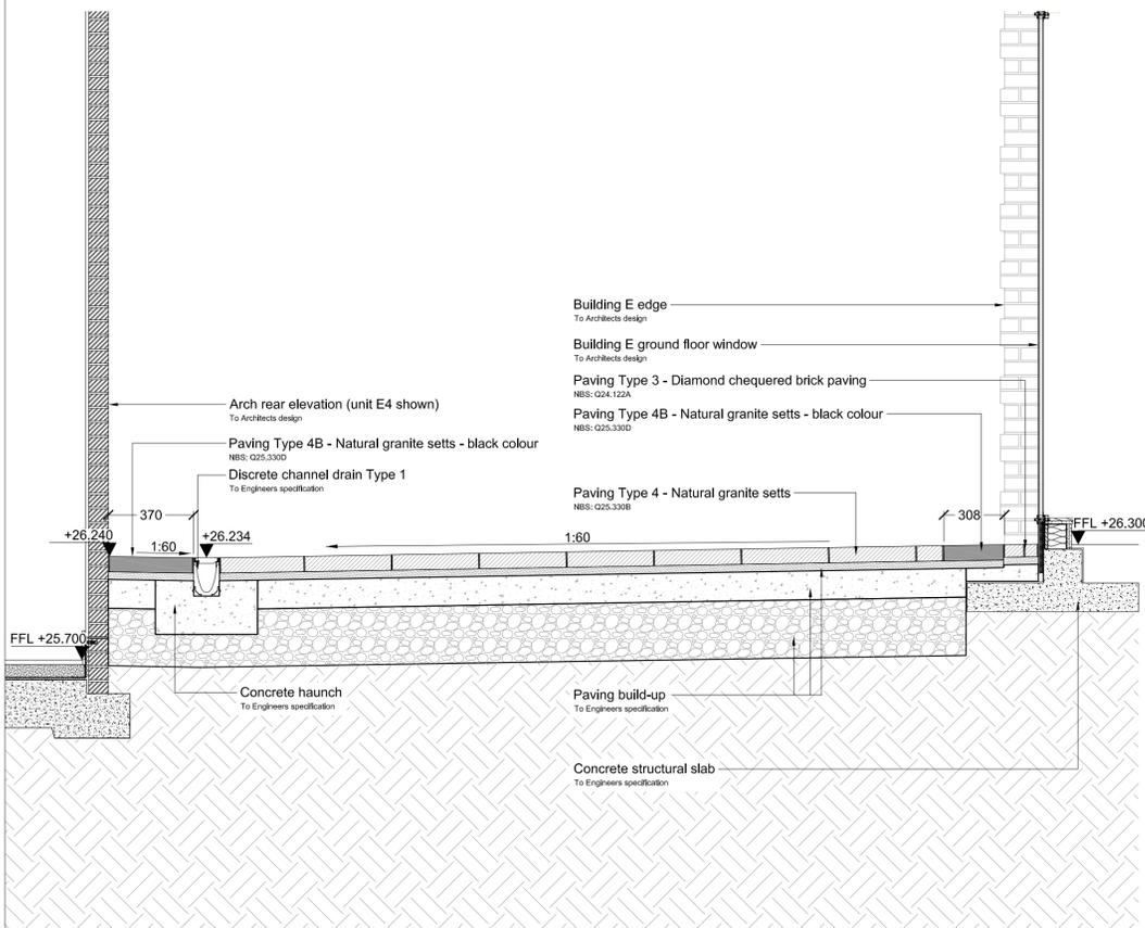
**8** Section through viaduct retail unit and building E ground floor windows
