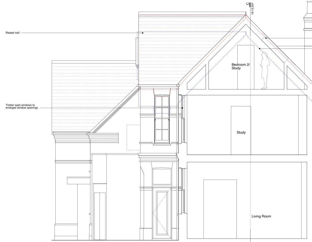
Rev.E 12.04.18: Blue broken line added to denote existing roof level Rev.D 23.02.18: Minor adjustments to rooflight sizes to suit supplier's details Rev.C 13.02.18: Roof level raised by 2 brick courses (c.150mm; intermediate glazing bars added to sash windows; door canopy added Rev.A 28.03.17: Rooflights amended.
