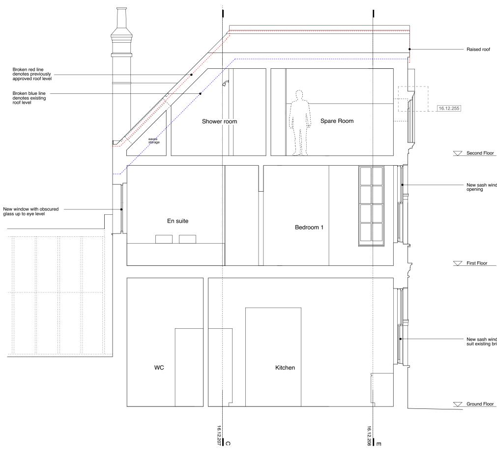
Rev.E 12.04.18: Blue broken line added to denote existing roof level Rev.D 23.02.18: Minor adjustments to rooflight sizes to suit supplier's details Rev.C 13.02.18: Roof level raised by 2 brick courses (c.150mm); intermediate glazing bars added to sash windows. Rev.A 28.03.17: Rooflights amended.
