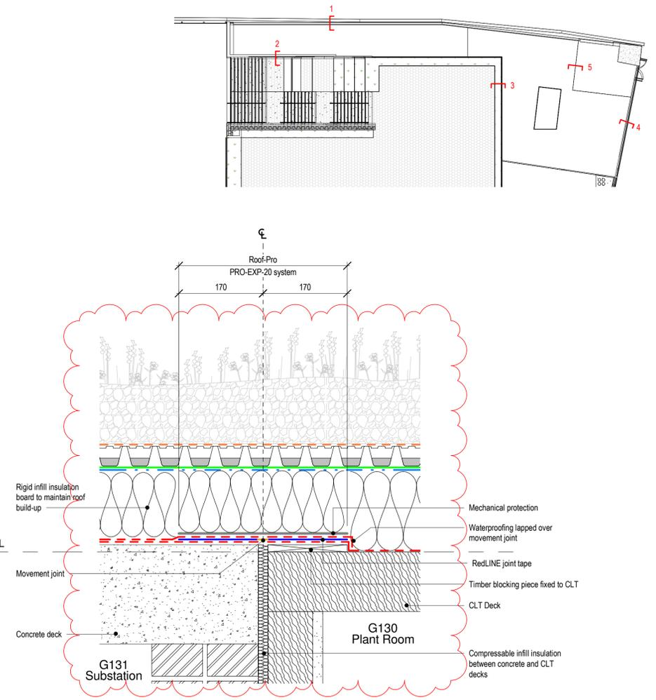
**5. Concrete Slab to CLT Slab**
