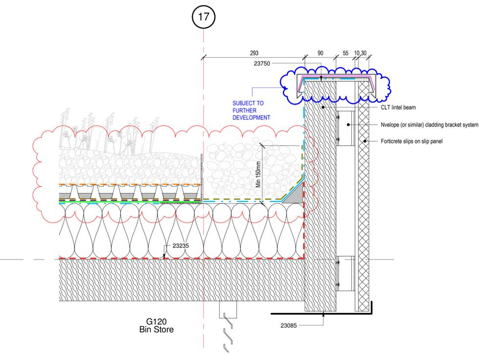
**4. GL 17 Lintel beam detail**
