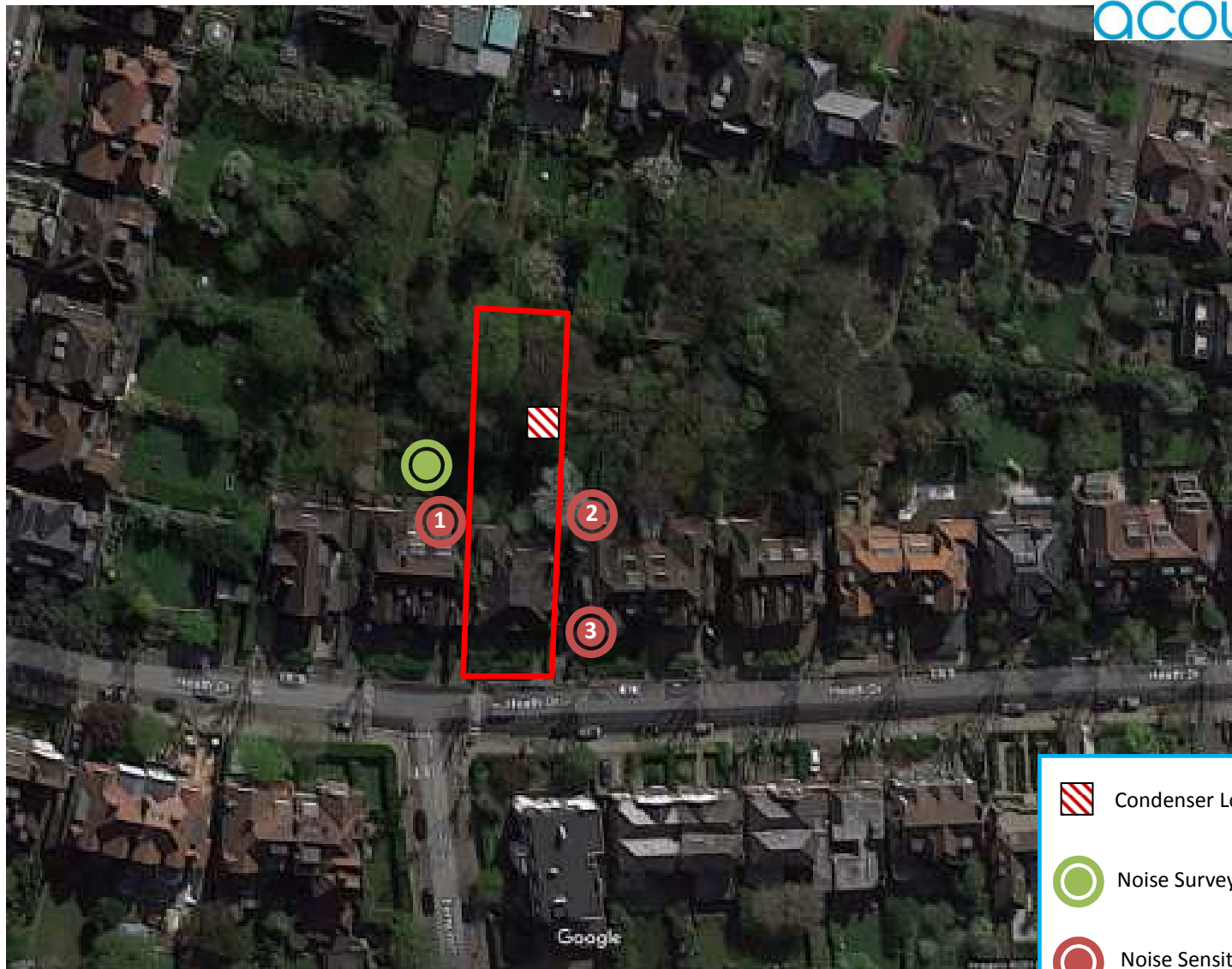
12935-SP1 Indicative site plan indicating noise monitoring position and nearest noise sensitive receiver
